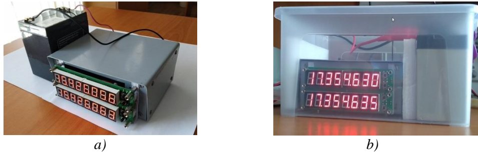
Fig. 1. Differential capacitance sensor in metal case (a) and hermetic container (b).
