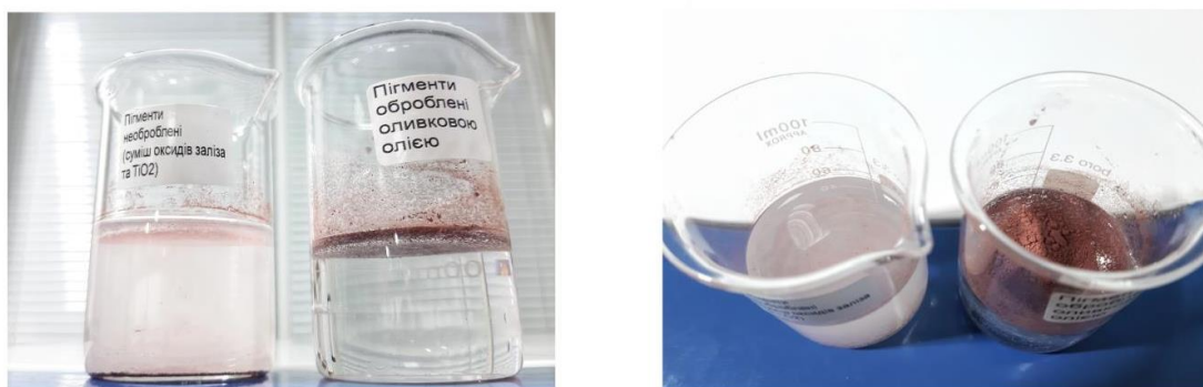
Fig. 3. The results of hydrophobicity of the mixture with untreated pigments \text{TiO}_2 and iron oxides and olive oil surface-treated mixture.
