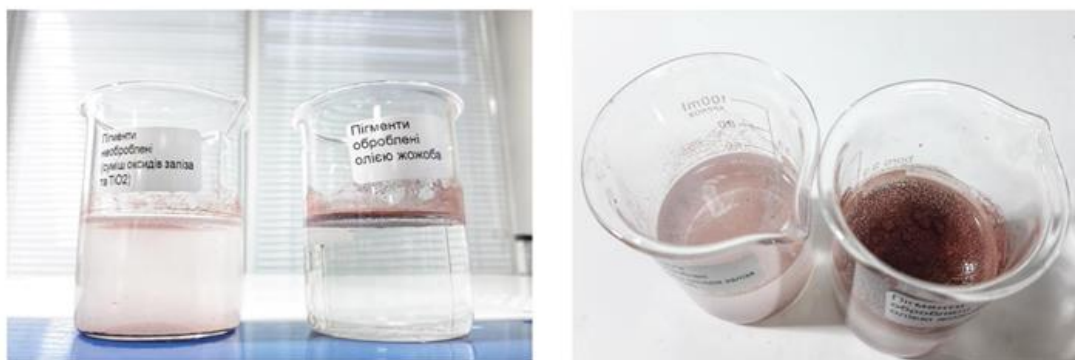
Fig. 4. The results of hydrophobicity of the mixture with untreated pigments TiO_2 and iron oxides and jojoba oil surface-treated mixture.
